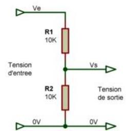
$$V_s = V_e * (R_2 / (R_1 + R_2))$$
